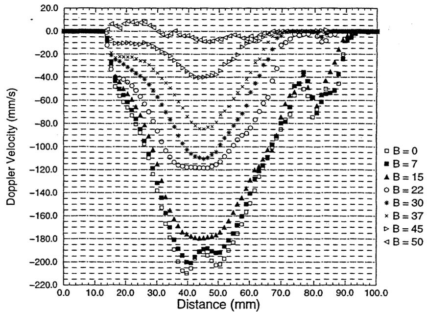
FIG. 2 - Direct measurements of velocity using the DOP 1000 multigate in a vortex of liquid Gallium for different magnetic fields (values in mT)
