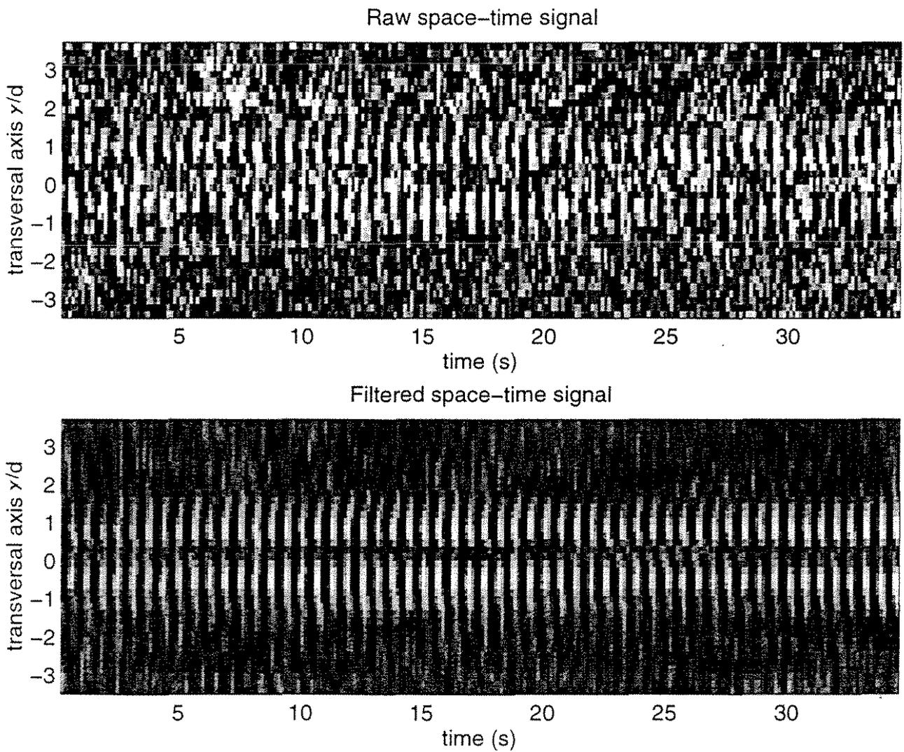
Figure 7: Spatio-temporal diagram of the transversal velocity component ( $R=120$ ,  $x/d=2$ ), gray scale coding of the velocity, a) raw data, b) filtered data. Note the sinuous mode of vortex shedding.
