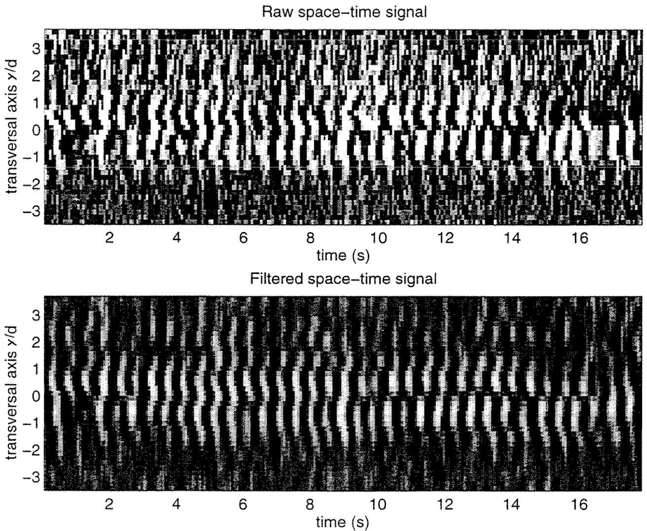
Figure 8: Space time diagram of the transversal velocity component ( $R=150$ ,  $x/d=3$ ), gray scale coding of the velocity, a) raw data, b) filtered data. Note the mixing of varicose and sinuous mode of vortex shedding.
