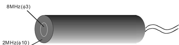
Figure 1: Schematic diagram of a multi-wave TDX.
