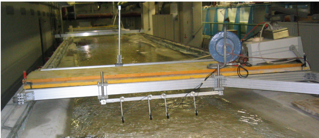
Figure 4: UVP transducers mounted on the measurement platform supported itself by rails
