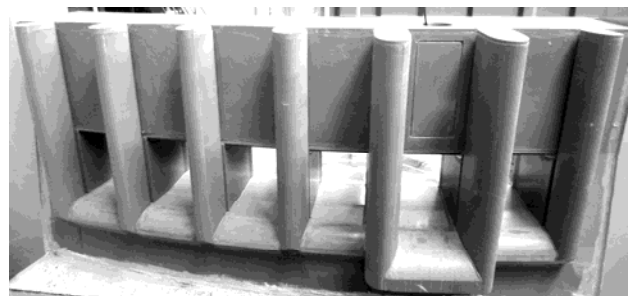
Figure 1: Physical model of orifice spillway seen from reservoir, considered gate is second from right
