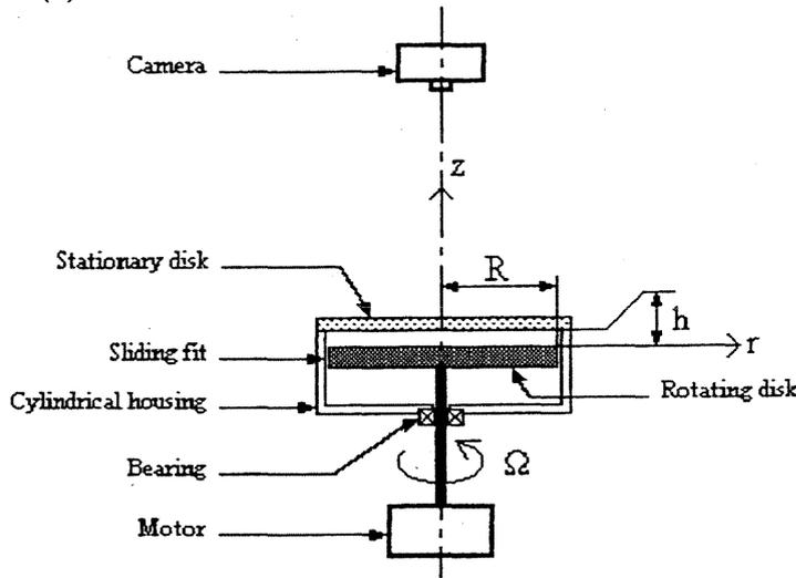
Figure 1: Experimental apparatus
