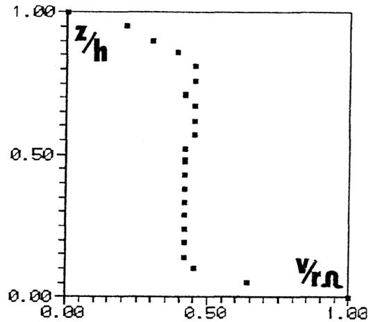
Figure 2: The Batchelor velocity profile of the rotating disk flow.  $Ek^{-1}=48$ ,  $Re=930$ .
