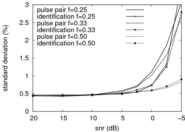
Figure 5: Comparison of the standard deviation at different frequencies.
