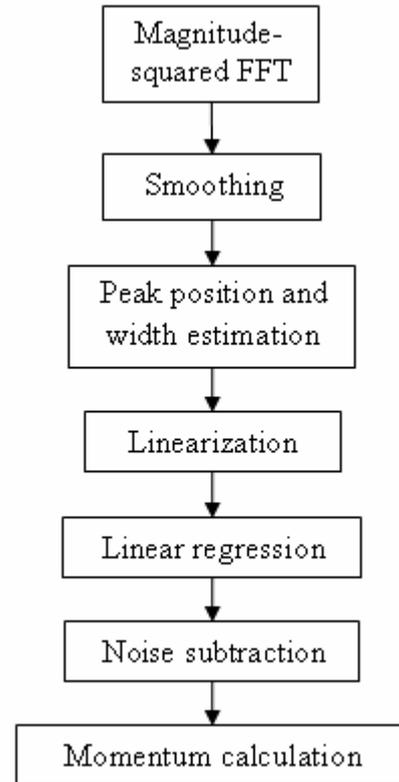
Figure 1: Steps of the spectral estimation method
