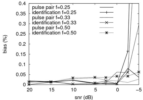
Figure 4: Comparison of the bias at different normalized frequencies.
