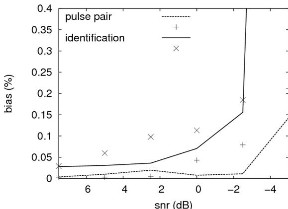
Figure 2: Comparison of the bias for the two methods with experimental data (points) and simulated data (lines).
