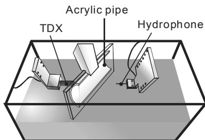
Figure 2: Schematic diagram of a experimental apparatus of ultrasonic intensity distributions at back of an acrylic pipe.
