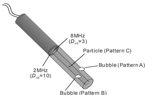
Figure 4: Schematic diagram of two-phase flow measurement using the multi-wave TDX.
