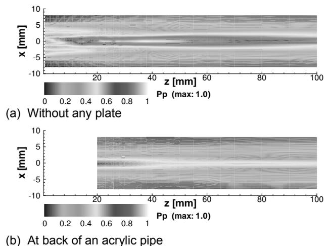
Figure 3: Measurement results of ultrasonic intensity distributions in 2 MHz of multi-wave TDX.
