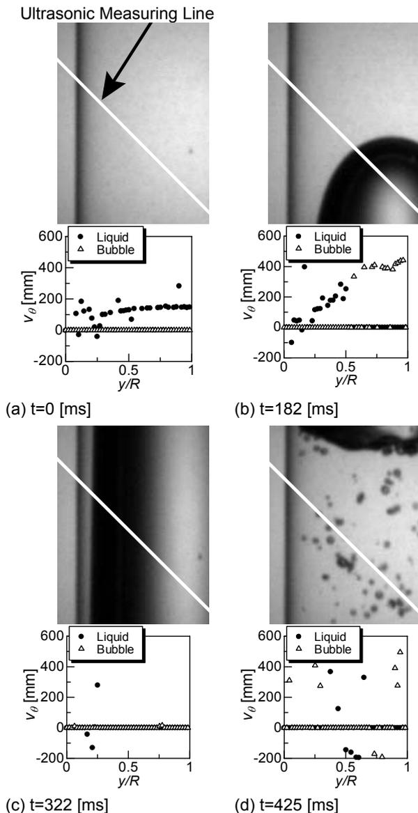
Figure 6: Pictures and velocity distributions of slug flow by using ultrasonic and high-speed camera.
