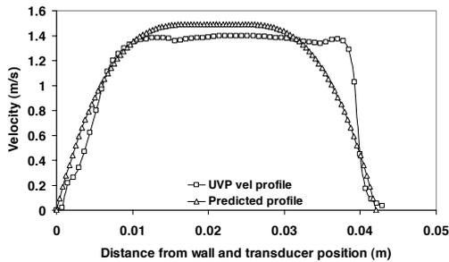
Figure 6: Velocity profile in 42 mm pipe for kaolin at flow rate of 1.3 l/s.
