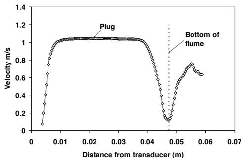
Figure 7: Velocity profile in 75 mm wide flume for Bentonite at flow rate of 2.26 l/s.
