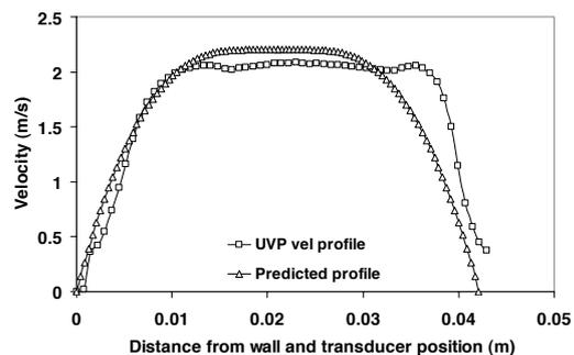
Figure 5: Velocity profile in 42 mm pipe for kaolin at flow rate of 1.9 l/s.
