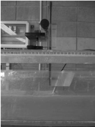
Figure 3: The 4 MHz probe fitted to the flume.
