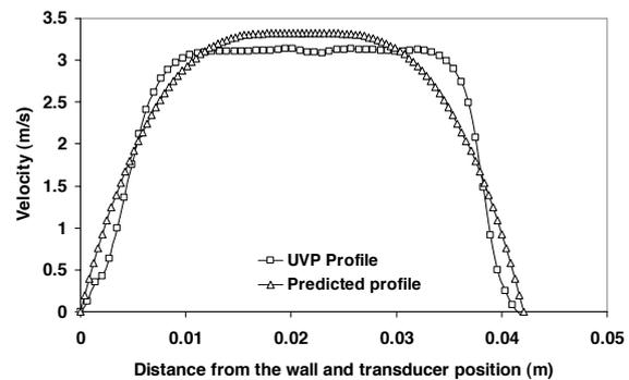
Figure 4: Velocity profile in 42 mm pipe for kaolin at flow rate of 2.8 l/s.
