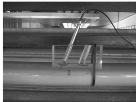
Figure 2: The 4 MHz probe fitted to the 40 mm pipe.
