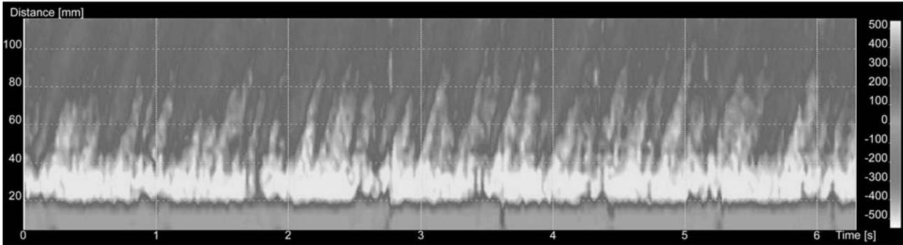
Fig.4: Space-time representation of the time dependent 1D velocity profile, where velocity condition is  $U_1$ .
