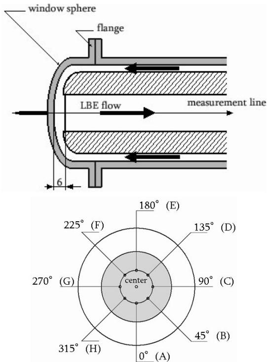
Fig.2: Experimental configuration of the measurement line on the window sphere
