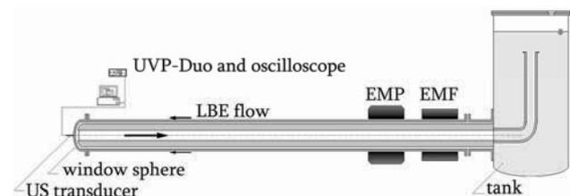
Fig.1: Experimental set-up and schematic illustration of JLBL-2.
