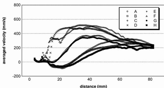
Fig.5: Averaged velocity profiles measured around the centerline of the measurement window at even intervals of angle, where measurement position labeled with A to G are expressed in Fig.2 (b) and velocity condition is  $U_1$ .
