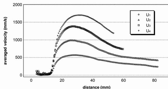
Fig.3: Averaged velocity profile at the centerline of JLBL-2, where velocity conditions are  $U_1, U_2, U_3, U_4 = 0.25, 0.50, 0.75, 1.00$  m/sec
