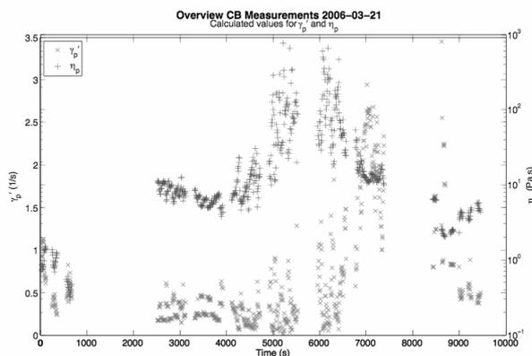
Figure 10: Calculated shear rates  $\dot{\gamma}_p$  and viscosity  $\eta_p$  for the plug.
