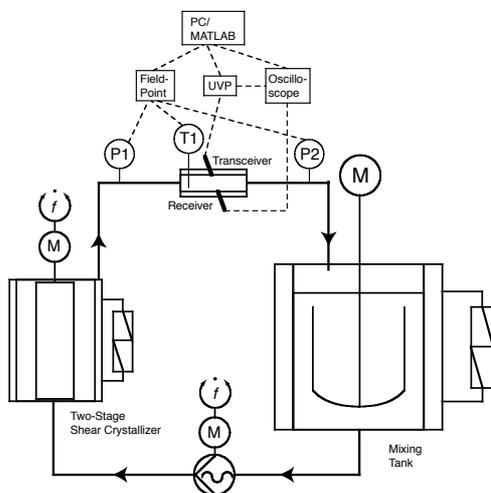
Figure 1 Scheme of the crystallizer flow loop, its instrumentation and data acquisition devices. P1, P2: pressure transducers; T1: thermocouple; M: motor; f: frequency transformer.
