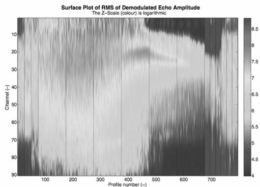
Figure 3: Surface plot of the root mean square of the demodulated echo amplitude with a logarithmic scale in Z (Color) direction. The measurement blocks are marked with vertical lines.
