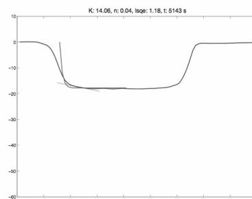
Figure 6: Measured (full curve) and fitted (half curve) velocity profiles after 5143 s (crystal suspension).
