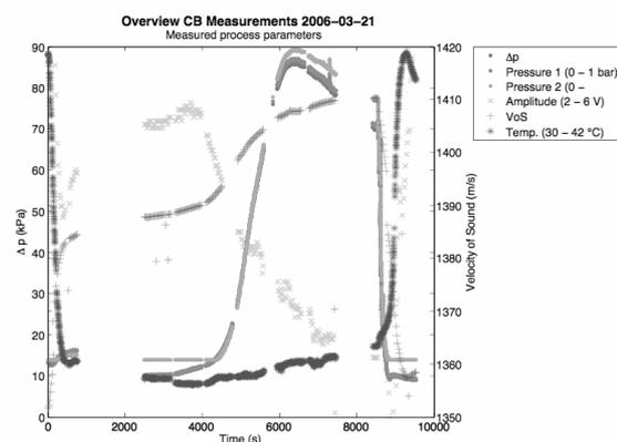
Figure 2: Overview for all the measured values of the crystallization process.
