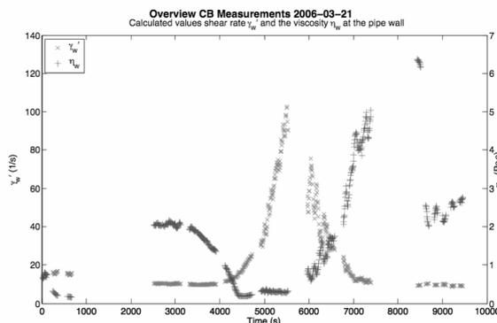
Figure 8: Calculated shear rates ( $\dot{\gamma}_w$ ) and viscosity ( $\eta_w$ ) at the wall.
