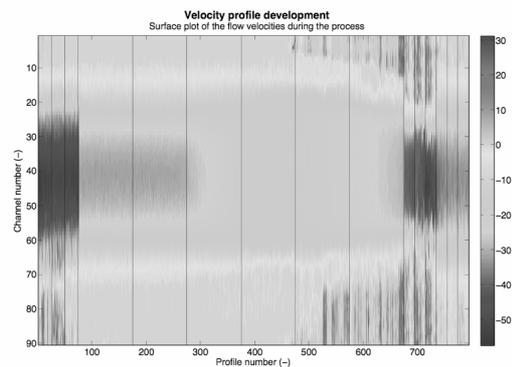
Figure 4: Surface plot of the flow velocities during the crystallization process. The development of velocity profiles along the diameter of the pipe is shown in Figures 6.64 and 6.65 during the three phases of the variation in process conditions.
