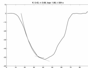
Figure 5: Measured (full curve) and fitted (half curve) velocity profiles after 564 s (liquid cocoa butter).
