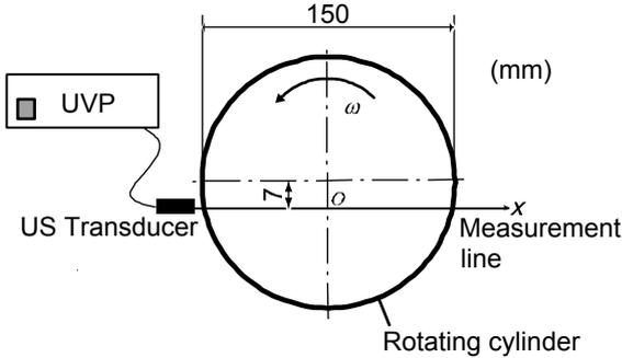
Figure 1: Definition of measurement line in container
