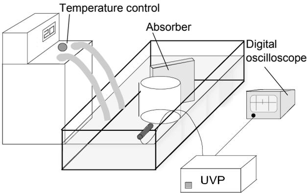
Figure 2: Experimental setup for PAA solution
