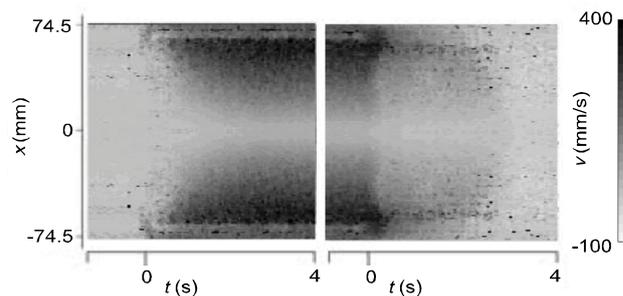
Figure 5: Spatio-temporal distribution of  $v$ , tangential velocity component.
