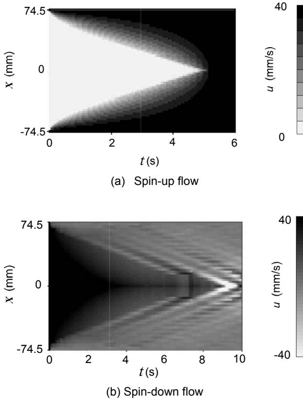
Figure 3: Spatio-temporal two-dimensional velocity distribution of visco-elastic fluid obtained by numerical simulated with Bingham model at 50rpm
