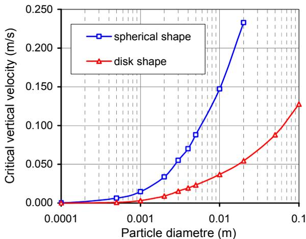
Figure 3: Critical velocity for frazil ice particle entrainment.
