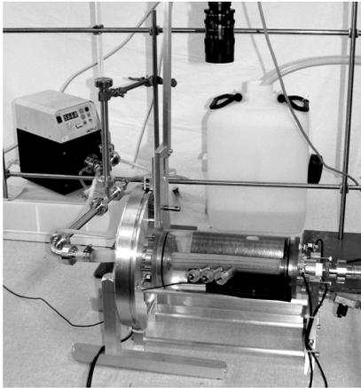
Figure 1: Ultrasound Doppler velocimetry for flow through collapsible silicone elastic tube in Starling resistor setup.
