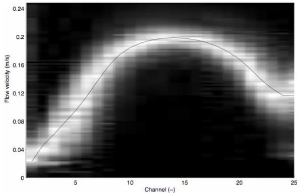
Figure 3: Velocity profile (full line: average profile) in collapsed elastic tube at 85 mbar external chamber pressure.
