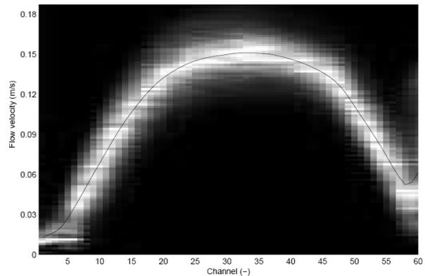
Figure 2: Velocity profile (full line: average profile) in undeformed elastic tube at 0 mbar external chamber pressure.
