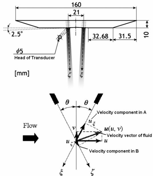
Figure 4: Y-type Angle Beam Transducer (2MHz)
