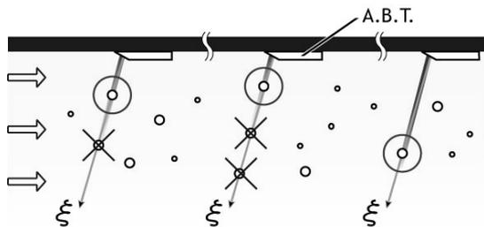
Figure 2: Ultrasonic beam reflection on nearest bubble
