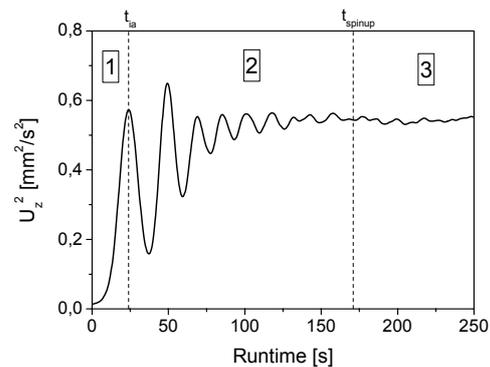
Figure 2:  $U_z^2$  averaged over the vertical velocity profile, obtained at a radial position of  $r/R_0 = 0.9$  and a magnetic field strength of  $B_0 = 0.42$  mT (1 – initial adjustment phase, 2 – inertial phase, 3 – steady state).
