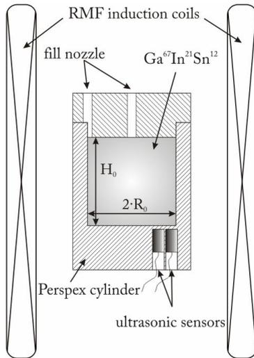
Figure 1: Schematic view of the experimental set-up
