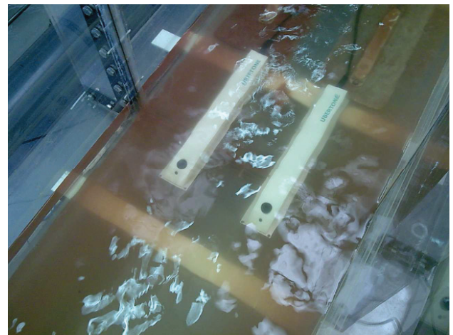
Figure 3: Two UB-Flow's placed in the flume
