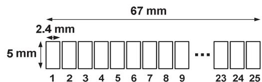
Figure 1: Design of a linear transducer array
