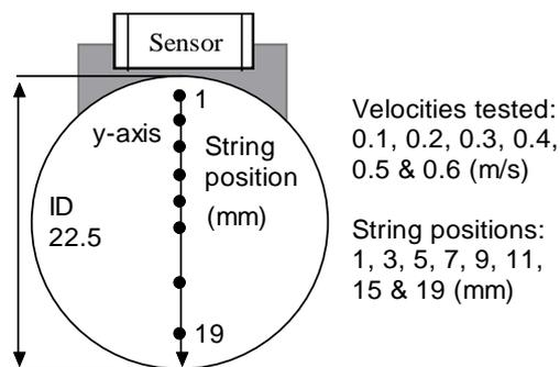
Figure 2: String positions and velocity range tested.
