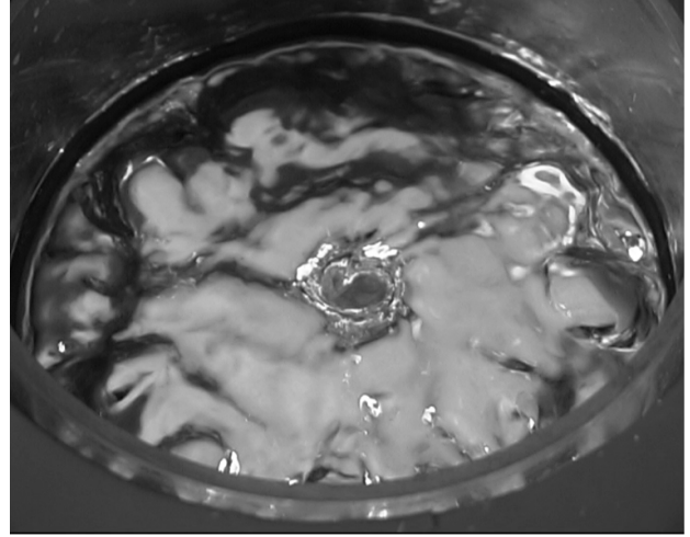
Figure 2: Snapshot of the free surface showing the tornado-like vortex funnel. D_0 = 170 mm; t = 1,8 s; Ta = 1.4 \times 10^7 ; F = 10^{10}
