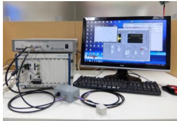
Figure 7: The measurement system developed for the steam jet flow measurement.
