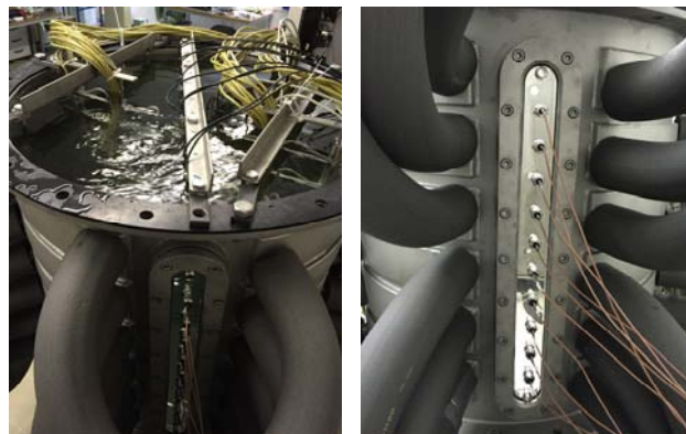
Figure 3: Cylindrical Part of the new modular tank with the temperature measuring grid and the arrangement of transducers
