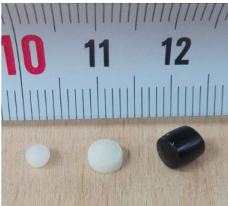
Figure 1: Picture of three tested fractions of plastic sediments – from left to right HSF30, TLT25, TLT50.
