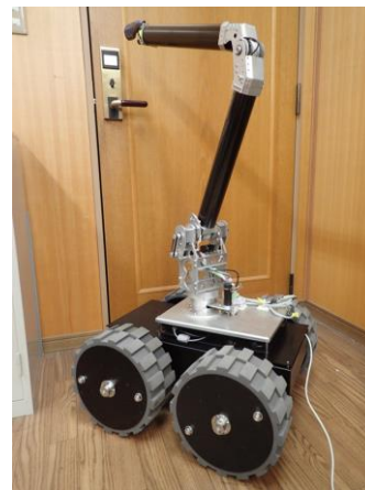
Figure 6: RhinoUS-I, a mobile manipulator with ultrasonic sensors
