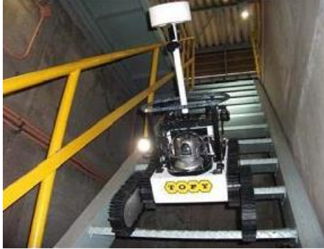
Figure 3: Survey Runner developed by TOPY Industries, Limited. ( http://www.topy.co.jp/release/201203/entry396.html )
