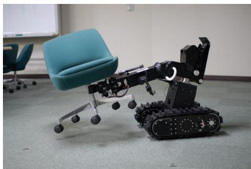
Figure 2: Helios IX lifting a 7kg chair
