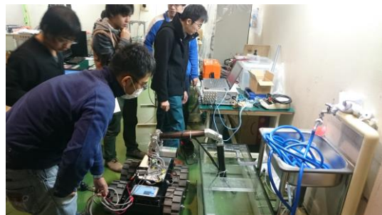
Figure 7: Students measured water flow in a tank by using ultrasonic sensors. Robot location and arm posture were remotely controlled by the students.
