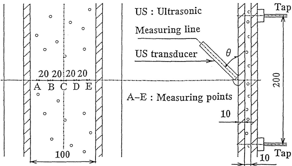
Fig.2 Test section
