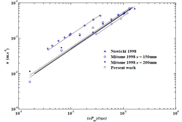
Figure 4: Comparison of present and former experimental data with the scaling law given from equation (3). The data from the literature are from Nowicki *et al.* [5] and Mitome [6].
