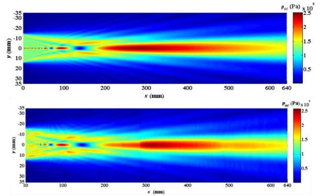
Figure 2: Iso-values of the acoustic pressure amplitude emitted by a circular plane transducer, issued from our linear propagation model (top) and experimental measurements (bottom).
