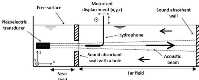
Figure 1: Sketch of the experimental configuration. The origin of the frame will be taken at the center of the acoustic source. The hydrophone is removed when PIV measurements are performed.
