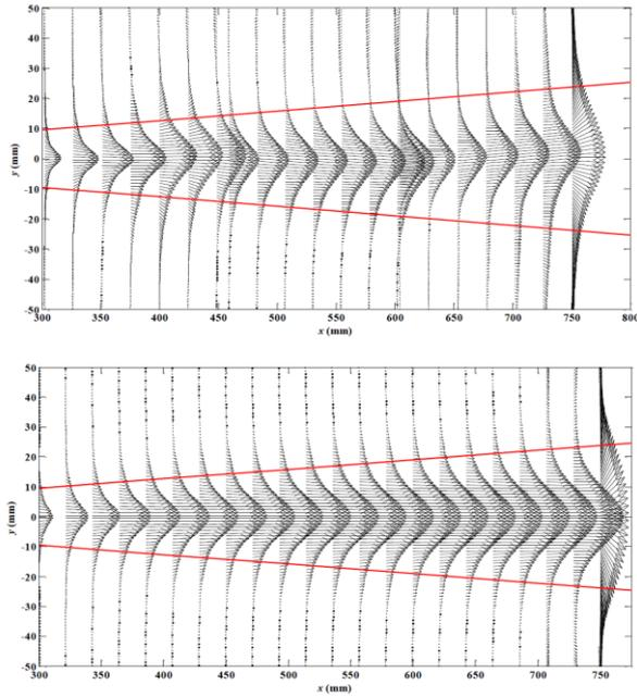
Figure 3: Typical velocity field, in the far field, issued from PIV measurements in the experiment (top) and from a numerical simulation (bottom). The red lines give the shape of the acoustic beam.
