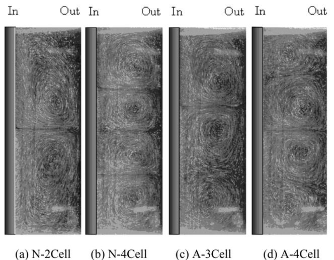
Fig. 4 Vortex mode at  $\eta=0.375$  ( $Re=370$ )
