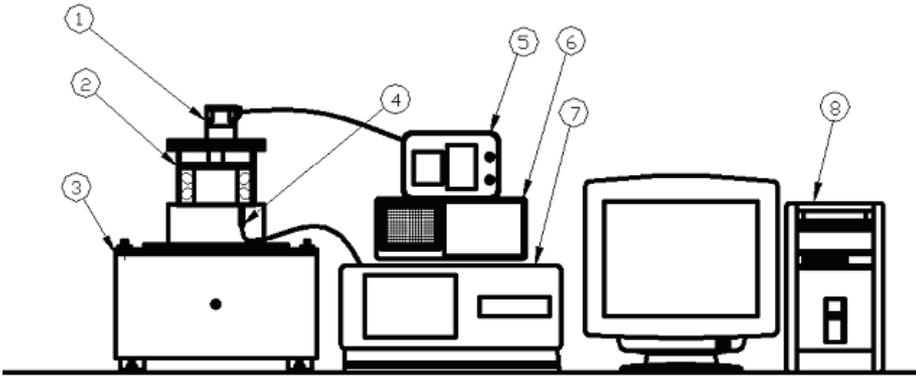
1.Motor, 2.Taylor-Couette Vessel, 3.Isolator, 4.US transducer, 5.Controller, 6.Oscilloscope, 7.UVP monitor, 8.Personal Computer
