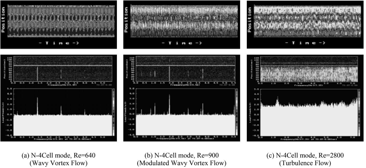
Fig. 5 Velocity fields and the corresponding space-averaged power spectra at  $\eta=0.667$
