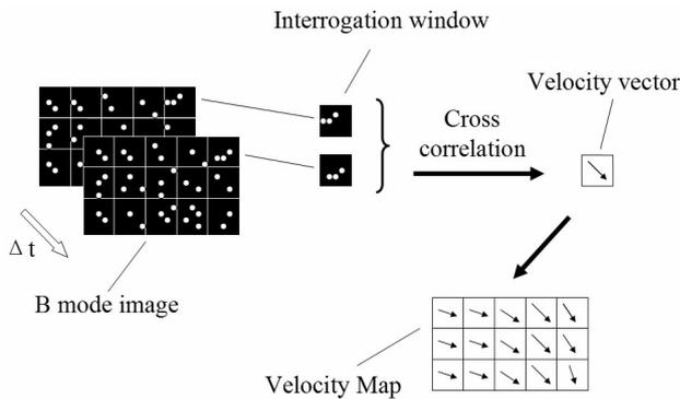
Figure 1: Schematic of the Echo PIV technique
