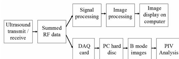
Figure 2: Data path schematic.
