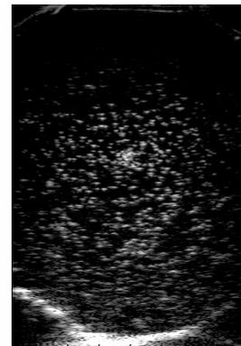
Figure 5: Echo PIV (B-mode) image of dilute contrast agent in a rotating flow.
