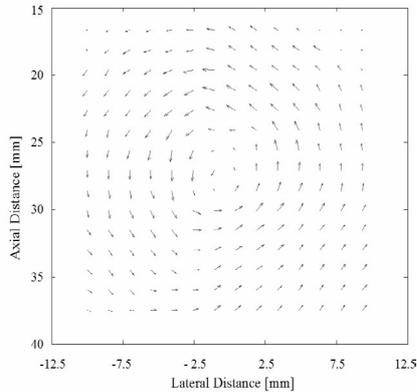
Figure 6: Velocity vectors resulting from Echo PIV processing of the image in Fig. 5.
