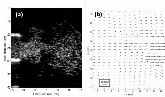
Figure 7: Jet flow measurement using Echo PIV: (a) B-mode particle imaging of the whole flow field; (b) Velocity field of the vortex ring at the head of the jet.
