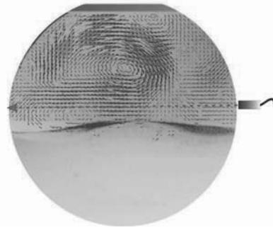
Figure 8: Velocity profile in cross section transverse to the pipe axis. The position of the UVP probe is indicated at the right. The image grayscale is inverted for clarity
