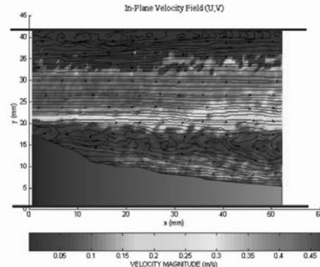
Figure 4: Development of shear layer between the main flow and the recirculation zone. The direction of the flow is from left to right. Flow rate is 0.2 l/s.
