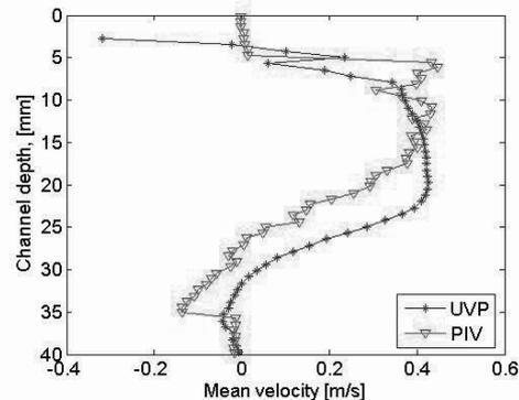
Figure 11: Direct comparison of UVP and PIV estimate, calculating the PIV component along the ultrasonic beam.
