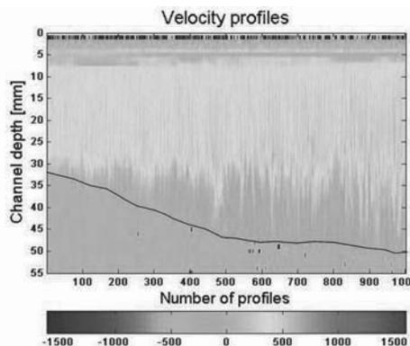
Figure 5: UVP velocity profiles above the dune. The UVP transducer is placed streamwise on top of the pipe at 12° from horizontal. The flow direction is from left to right. Mean flow velocity U = 0.18 m/s. Colorbar in mm/s.
