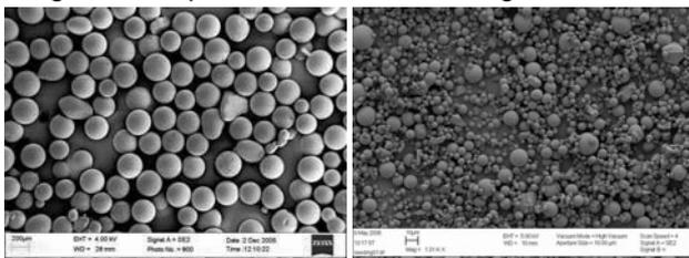
Figure 3: SEM pictures of bed particles (left) and seeding particles (right).
