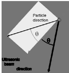
Figure 10: The axial symmetric nature of the UVP measurements may cause different particle directions to yield the same velocity component.
