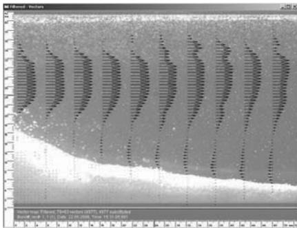
Figure 6: A close-up of an example of the axial velocity profile superimposed on the picture of the sand dune. The flow direction is from left to right. The image grayscale is inverted for clarity.  $U = 0.18$  m/s.
