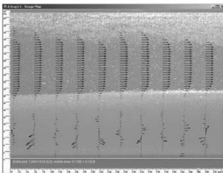
Figure 7: PIV velocity profiles above the dune stoss. The flow direction is from left to right. The image grayscale is inverted for clarity.  $U = 0.22$  m/s.
