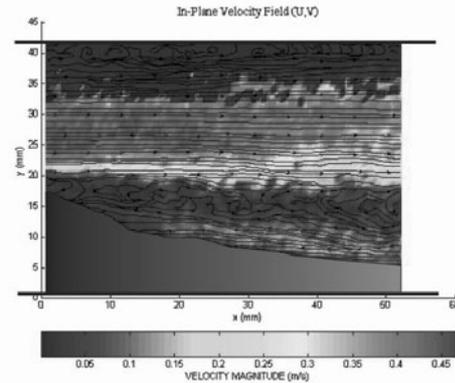
Figure 4: Development of shear layer between the main flow and the recirculation zone. The direction of the flow is from left to right. Flow rate is 0.2 l/s.
