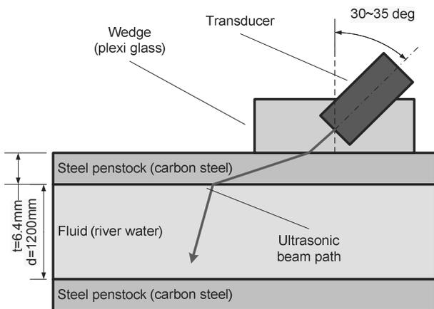
Figure 1: Schematic diagram of installation of ultrasonic transducer clamped on pipe surface
