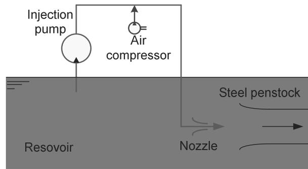
Figure 3: Configuration of bubble injection system to supply miniaturized bubbles as ultrasonic reflectors into steel penstock
