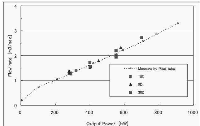
Figure 8: Comparison of flow rate vs. power output between Pitot tube and UdFlow at different horizontal diameter positions
