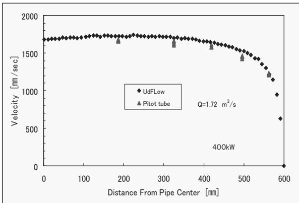
Figure 6: Comparison of velocity profile for 400kW between Pitot tube and UdFlow
