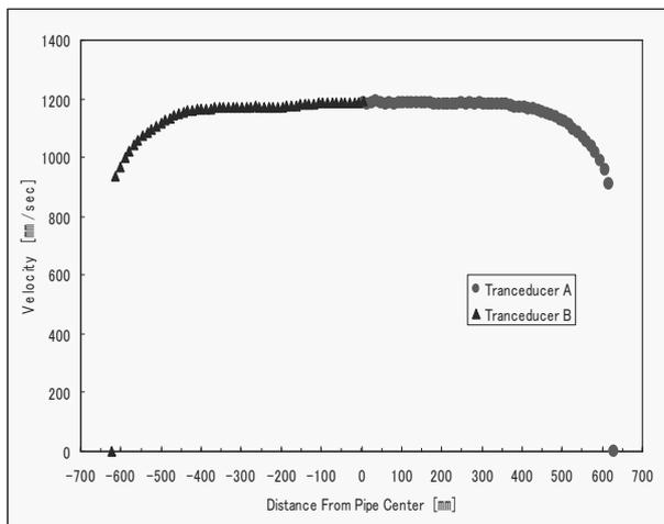
Figure 10: Velocity profiles obtained by multiline measurement method with two transducers placed at opposed circumferential positions on steel penstock
