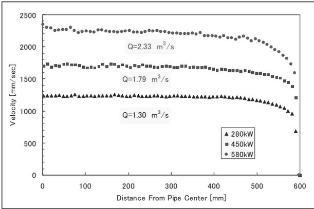
Figure 5: Velocity profiles for the different power outputs at the horizontal diameter position of 9D
