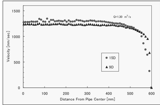
Figure 7: Velocity profiles for 280kW at the horizontal diameter positions of 9D and 15D
