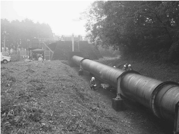
Figure 9: Measuring point of ultrasonic flowmeter at horizontal diameter position of 19D from the inlet of steel penstock at Okuragawa hydraulic power station
