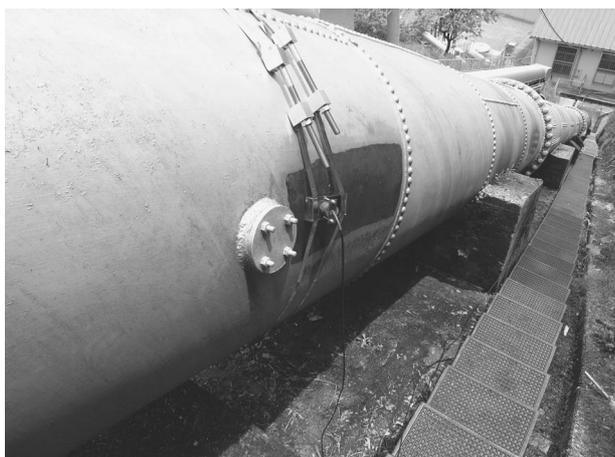
Figure 2: Ultrasonic transducer and wedge installed on the surface of steel penstock at hydraulic power plant
