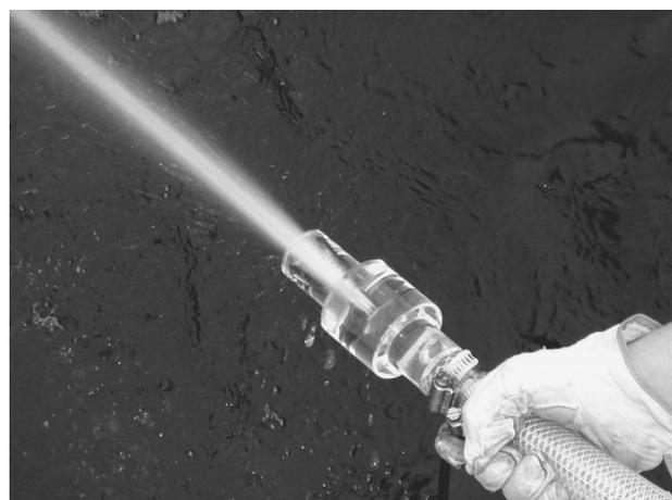
Figure 4: Water jet from injection nozzle to supply miniaturized air bubbles
