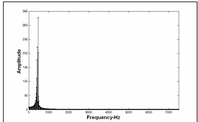
Figure 2: Spectrum of PUS received from center of pipe (ID=50mm) for velocity component in probe direction. Sampling frequency is 14346 Hz and sampling number is 1024. Local average velocity is 234 mm/s and it has an oscillating part with frequency 10Hz and amplitude 10% of the average.
