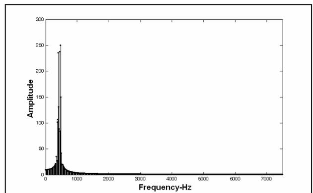
Figure 3: Spectrum of PUS received from center of pipe (ID=50mm) for velocity component in probe direction. Sampling frequency is 14346 Hz and sampling number is 1024. Local average velocity is 234 mm/s and it has an oscillating part with frequency 20Hz and amplitude 10% of the average.
