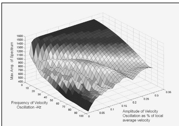
Figure 4: Change of maximum spectral amplitude P.U.S. with oscillating velocity components. Simulation parameters are: local average velocity is 0.234 m/s, , for the center of pipe with ID=50mm, Tpc (one profile measurement time)=0.2855 s (3.5 Hz).
