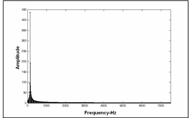
Figure 1: Spectrum of PUS received from center of pipe (ID=50mm) for velocity component in probe direction. Sampling frequency is 14346 Hz and sampling number is 1024. Local velocity is 78 mm/s without any fluctuation.
