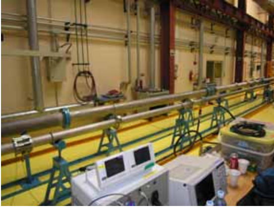
Figure 7 Layout of CENAM standard loop for water and pipe arrangement.
