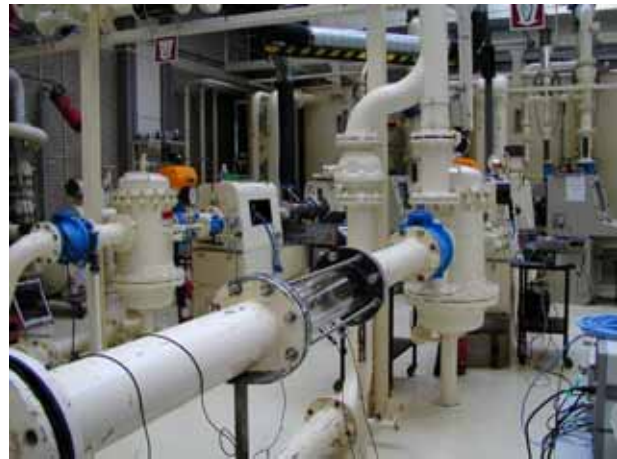
Figure 6. Layout of NMI standard loop for kerosene
