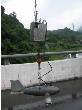
Figure 3: ADP, sounding and wireless communication unit.
