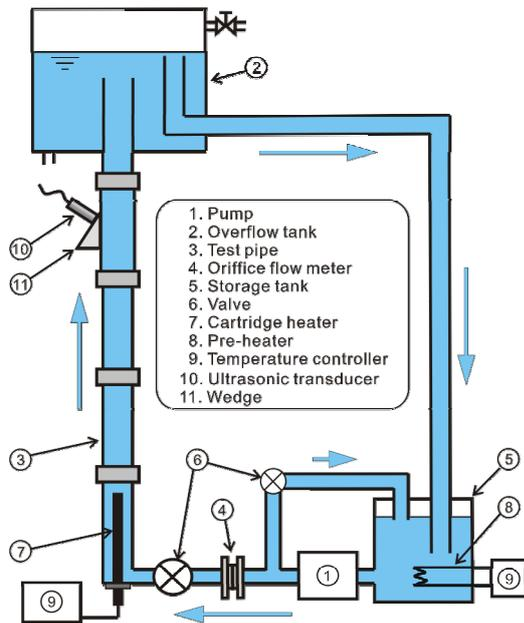
Figure 7: Schematic diagram of experimental loop for boiling two-phase flow measurement
