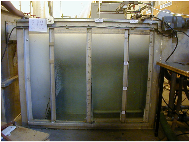
Figure 1. The pilot plant with hydraulic load and dispersion flow (bubbles) entering the riser shaft to the left
