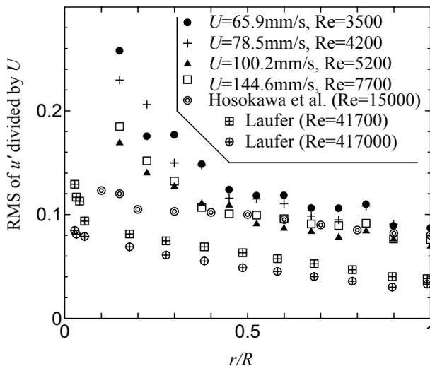
Figure 7: RMS value of velocity fluctuation  $\sqrt{u'^2}$  divided by the cross-sectional averaged flow velocity  $U$  measured by the UVP contact measurement ( $D=53.5\text{mm}$ ) together with existing data
