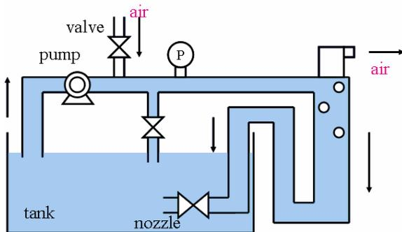
Figure 3: Micro bubble generator
