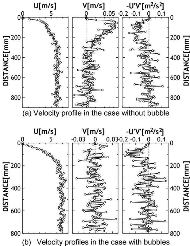
Figure 9: Velocity profiles (YABT-0.5MHz) at stern
