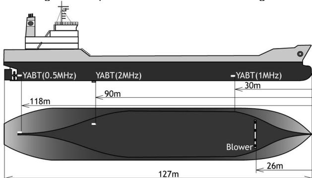
Figure 6: Mounting position of three different YABTs
