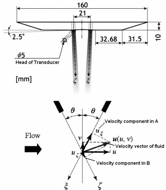
Figure 4: Y-type Angle Beam Transducer (2MHz)
