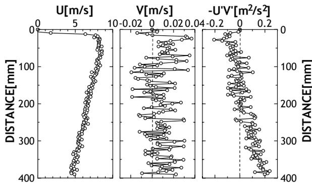
(b) Velocity profiles in the case with bubbles
