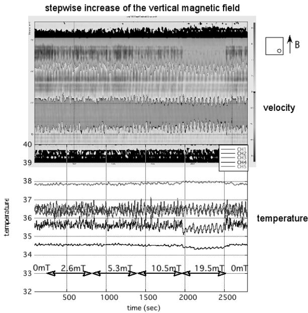
Figure 5: The behavior of the flow with stepwise increase of the vertical magnetic field.  $Ra=1 \times 10^5$ . 0 mT, 2.6 mT, 5.3 mT, 10.5 mT, 19.5 mT, and again 0 mT, is the intensity of the imposed vertical magnetic field. Typical flow velocity is decreasing with the increase of magnetic field, though it is not clear in this grayscale. Note that the total time in this series is longer than in Figure 4.
