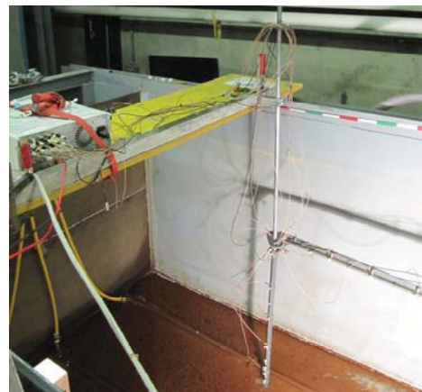
Figure 3: The 5 \times 5 UVP-transducers rack fixed on the vertical stem with its remote computer installed on the bridge.
