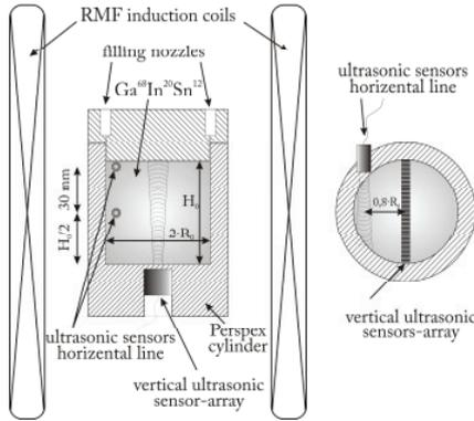
Figure 1: Schematic view of the experimental setup
