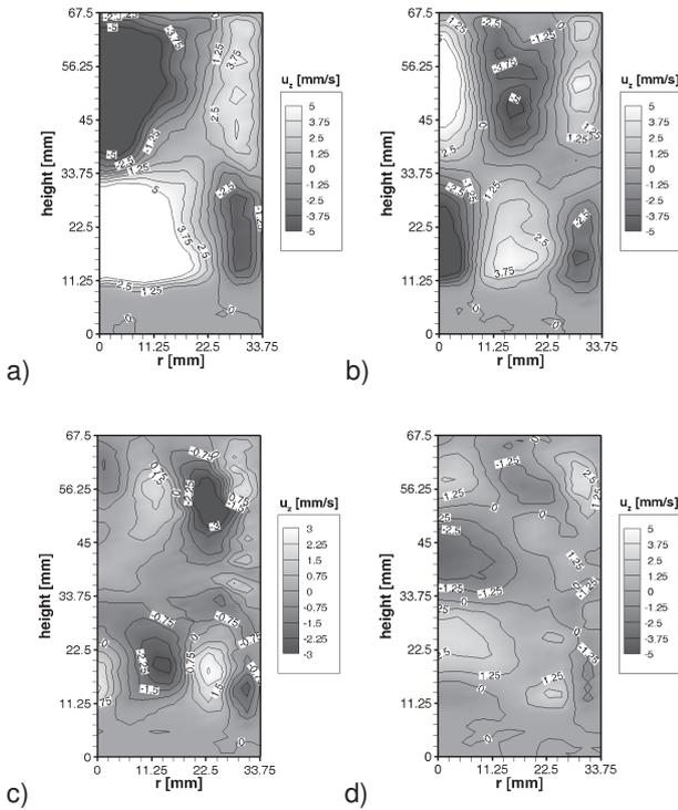
Figure 5: Snapshots of the vertical velocity across the vertical mid-plane of the cylinder recorded by the US sensor array at  $B_{RMF} = 2.25$  mT: (a)  $T_P = 2.95$  s, (b)  $T_P = 4.3$  s; (c)  $T_P = 5.3$  s and (d)  $T_P = 2.35$  s
