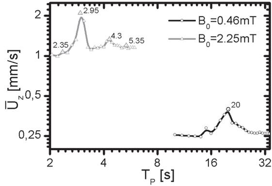
Figure 4: Dependence of the intensity of the secondary flow on the duration of the pulse cycle
