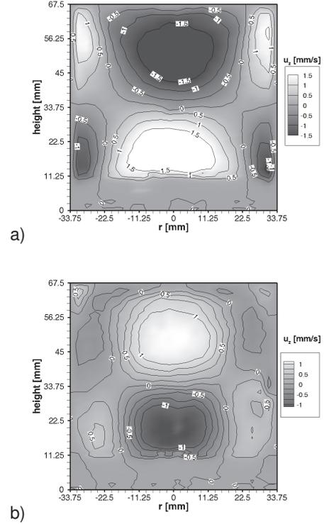
Figure 3: Snapshots of the vertical velocity across the vertical mid-plane of the cylinder recorded by the US sensor array for  $T_P = 20$  s at  $B_{RMF} = 0.46$  mT: (a) typical double vortex of the secondary flow; (b) “inverse” double vortex
