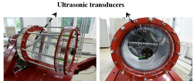
Figure 3: Photograph of the rotating cylinder and of the UDV sensors for the measurement of the axial velocity.
