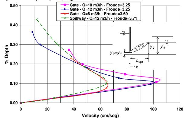
Figure 4: Velocity distributions in hydraulic jumps.
