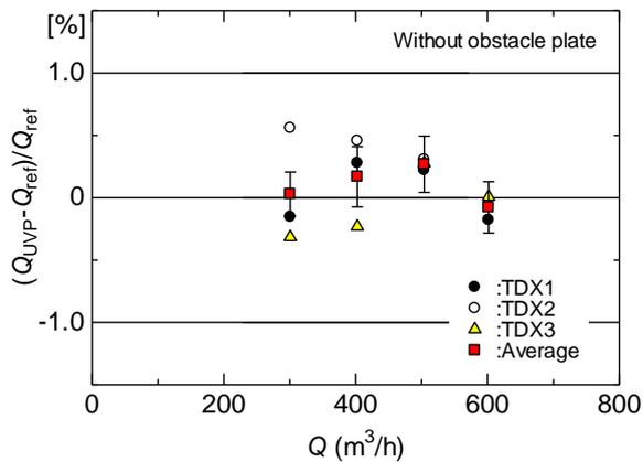
Figure 4: Deviation of flowrate given by ultrasonic Doppler method from reference by static gravimetric method for straight pipe without obstacle plate
