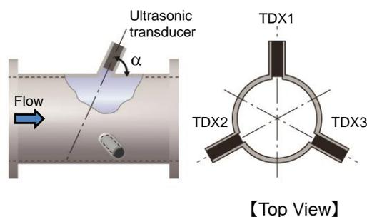
Figure 1: Test section
