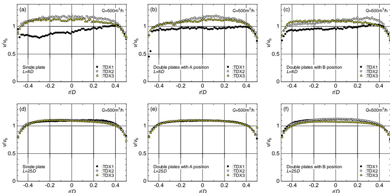
Figure 5: Velocity profiles downstream of obstacle plates
