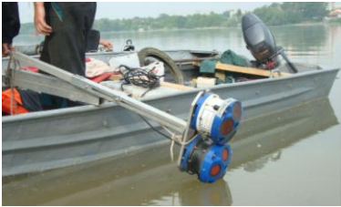
Figure 2: 1200- and 600-kHz ADCPs (by Teledyne RDI) installation at vessel side; inactive phase before looking-down actual deployment.
