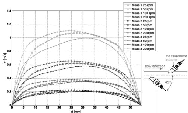
Fig. 4: Velocity profiles of the pipe flow at the horizontal test section of the LIMMCAST facility for different pump speeds.
