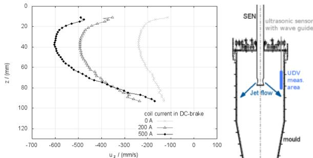
Fig. 5: Vertical velocity along the narrow mold wall (left) and sketch of measurement configuration (right).
