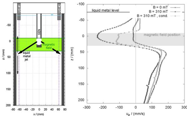
Fig. 3: Measurement configuration for mean vertical velocity along the narrow mold wall at the Mini-LIMMCAST setup (left) and corresponding results of one sensor for different experimental conditions (right).
