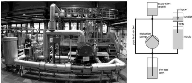
Fig. 1: LIMMCAST – large scale (250 °C) liquid metal experiment for continuous flow measurement in tundish, SEN and mold (left) and a schematic setup (right).
