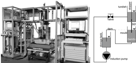
Fig. 2: Mini-LIMMCAST – small scale acrylic glass model for experimental flow investigations at room temperature using GaInSn (left) and a sketch of the operation principle (right).
