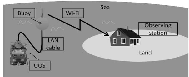
Figure 4: Schematic explanation of the operation of the Gyogyotto camera and the video delivery path.
