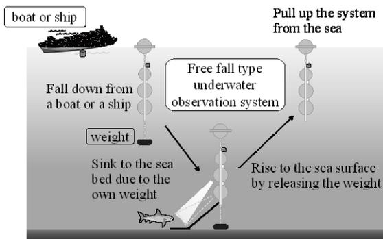
Figure 1: The operation of the free-fall type UOS.
