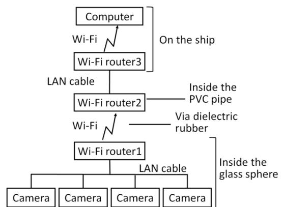
Figure 5: Diagram for delivering path of movie and data.
