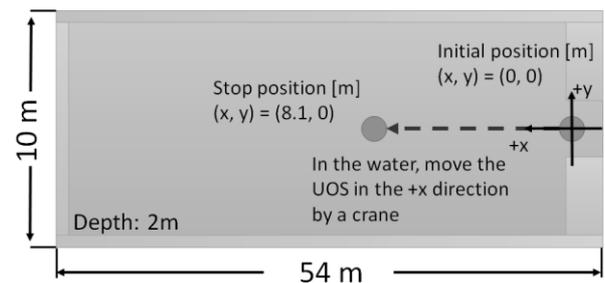
Figure 8: The setup for the position estimation experiment.
