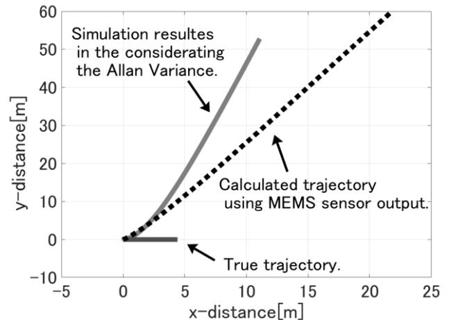
Figure 10: The UOS's trajectory under the water.
