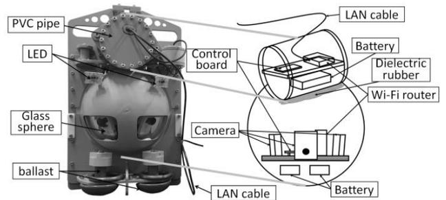
Figure 3: The configuration of Gyogyotto Camera.
