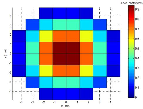
Figure 1: Transducer aperture geometry representation divided in 1.2 mm x 1.2 mm square mathematical elements. Apodization coefficients used for each element are also showed by color palette.
