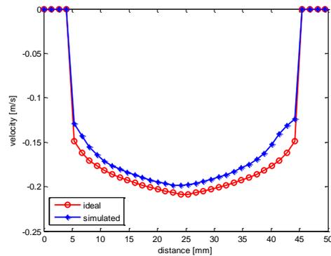
Figure 5: Spatial velocity profile measured versus spatial velocity profile simulated for turbulent flow where  $V_{max} = 0.8 v_a$ , SNR=50 dB,  $N_{pulse}=50$ .
