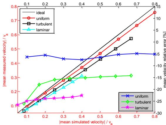
Figure 7: Left axis: Mean spatial measured velocity (cross-correlation) versus mean spatial simulated velocity, both normalized by the maximum velocity,  $v_a$ . Legend at top left. Right axis: mean velocity relative error for each flow and each simulated velocity. Legend at bottom right.
