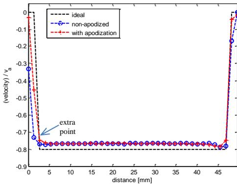
Figure 3: Comparison of velocity profile obtained from a non-apodized aperture with a velocity profile from an apodized aperture.
