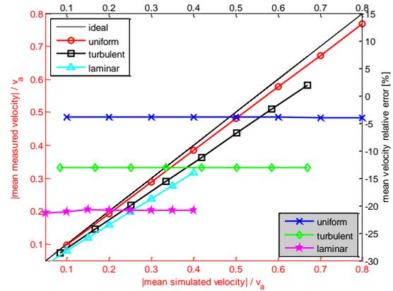
Figure 4: Left axis: Mean spatial measured velocity (autocorrelation) versus mean spatial simulated velocity, both normalized by the maximum velocity of the autocorrelation method,  $v_a$ . Legend at top left. Right axis: mean velocity relative error for each flow and each simulated velocity. Legend at bottom right.
