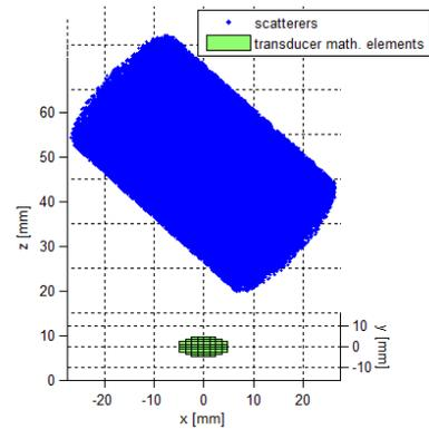
Figure 2: 3D representation of reflectors distribution with respect to the ultrasound transducer. Pipe walls were suppressed.
