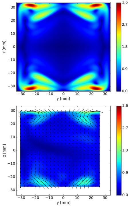
Figure 4: Mean velocity of the secondary flow in mm/s for  $Ta = 10^5$  (top: computed from the numerical simulation, bottom: measured mean velocity distribution)
