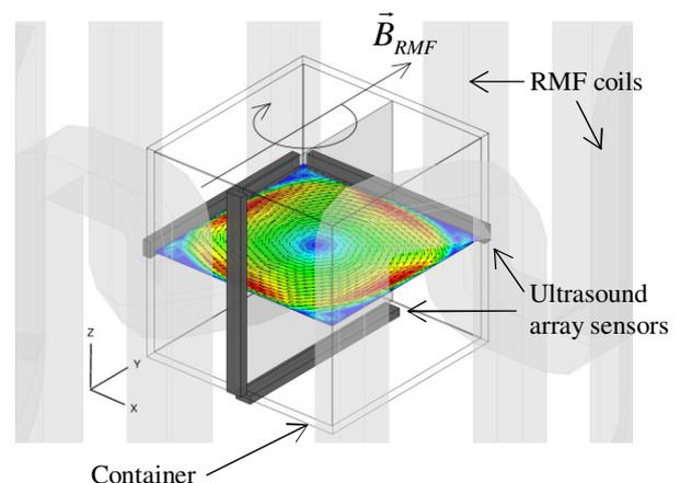
Figure 1: Measurement configuration: cube instrumented with four ultrasound array sensors.
