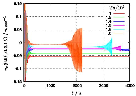
Figure 3: Time evolution of  $u_x$  at a monitoring point for different values of the magnetic Taylor number  $Ta$ .
