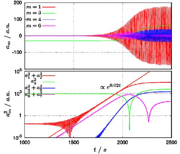
Figure 5: POD of the primary flow (numerical simulation for  $Ta = 1,7 \times 10^5$ ) - Time evolution of the amplitude of the most important modes  $a_m(t)$ ;  $m = 1, 3, 4, 6$  (top) and of the kinetic energy of the modes  $m = 1, \dots, 7$  (bottom).
