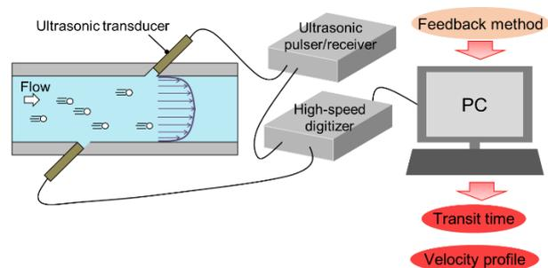
Figure 5: Schematic of the hybrid ultrasonic flow meter.
