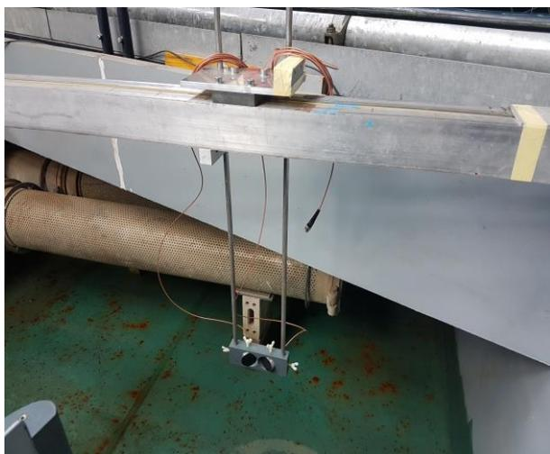
Figure 3 UVP sensors, frame and carriage
